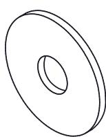
$\varnothing 16/\varnothing 5 \times 1$  mm
